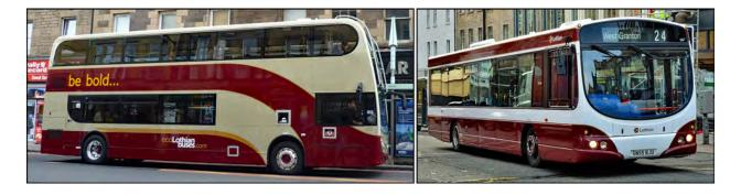
The Lothian Bus fleet includes diesel-electric, low-carbon "hybrid" buses (above, left), and fully electric single deck buses (above, right).
